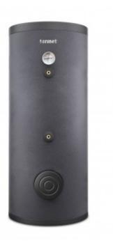
TERMET AQUA 200 I tanks (with a double coiled coil) are intended only for heating, storing and supplying hot water. The device is made of highquality steel, additionally internal anti-corrosion protection made by the enamelling process. An additional protective element is the protective anode, which is a consumable element and subject to cyclical mandatory replacement (see warranty conditions).
